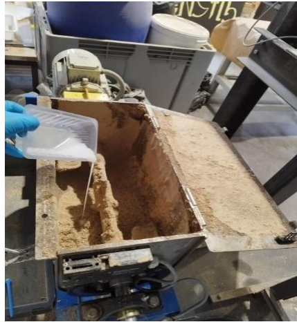
Figure 17: The gluing system used for particle boards production at lab scale
