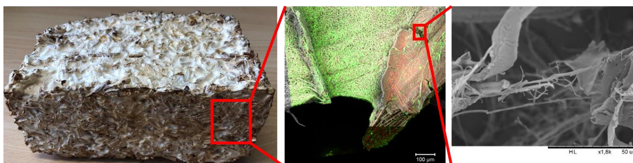
Figure 3: Multiscale visualization of a myco-composite material. From left to right : macroscopic view of a wood particles based myco-composite material glued with Trametes versicolor ; correlative microscopy (CLSM-SEM) showing the fungal hyphae in green and the wood in red; SEM detail showing hyphae connecting two wood particles.
