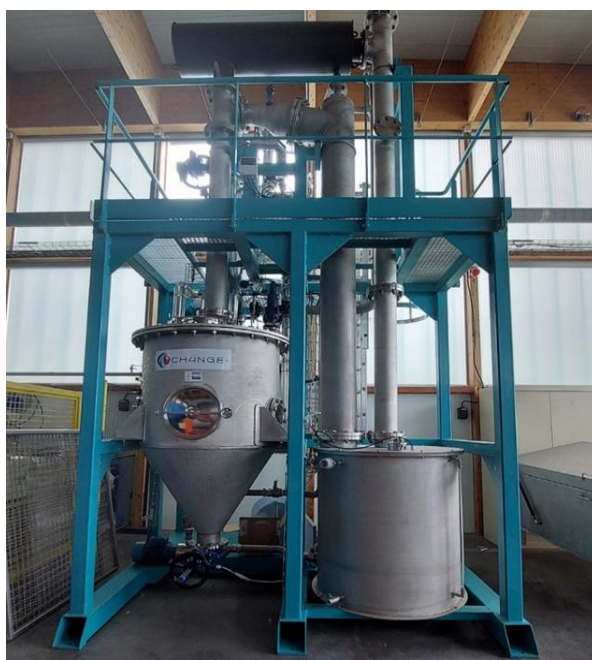
Figure 2: Steam explosion pilot at LERMAB (CH4NGE, France)
