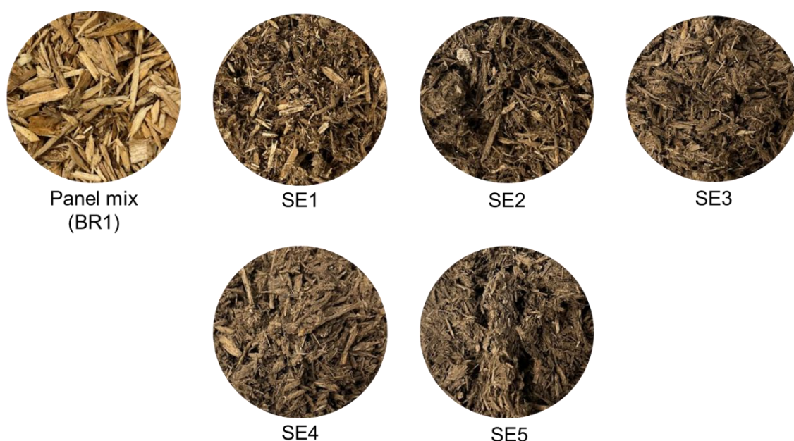
Figure 19. Macroscopic pictures of the panel mix after five cascading steam explosions in mild conditions.
