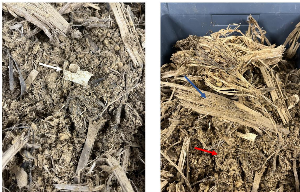
Figure 18. Particleboards and raw wood from the Ecomaison batch after steam explosion at high severity conditions. The biomass shows frayed fibers and ruptured wood fragments (blue arrows), fine fibrous particles from panel breakdown (red arrow), and detached melamine coating (white arrow).
