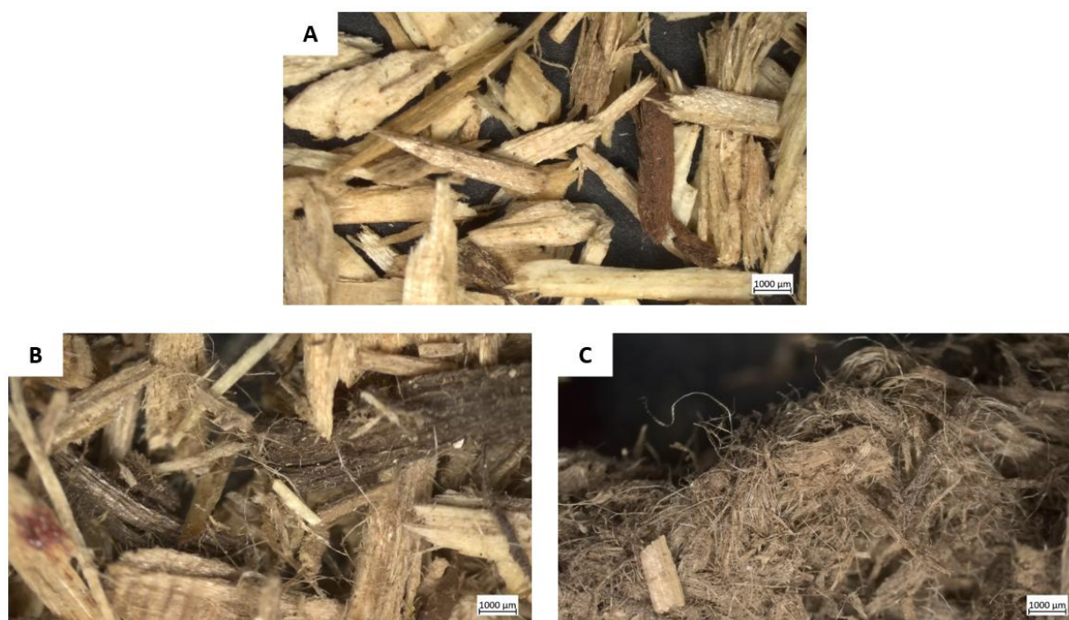
Figure 20. Binocular images of the Panel mix (A), steam-exploded sample SE1 (B), and steam-exploded sample SE5 (C).
