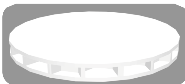
Figure 14. 3D-rendered image of the honeycomb-type panel.
