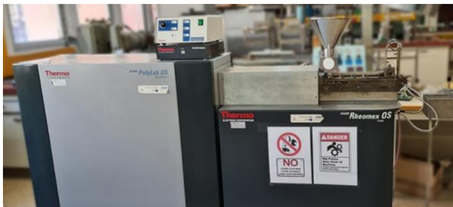
Figure 2. HAAKE Thermo Fischer PTW16 twin-screw extruder at NTUA LPT.
